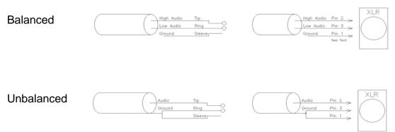
**Note:** When using balanced line, only one end of the line should be grounded. This will help avoid ground loops. As shown above, the ground would be connected at the 'send' end and not connected to the RM-35.
